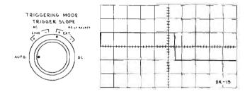
Fig. 2-1. Triggering on the rising portion of a waveform. The TRIG-GER SLOPE switch is at + EXT., so that the display starts during the positive-going part of the waveform (that is, during that part of the waveform where the slope is positive).
