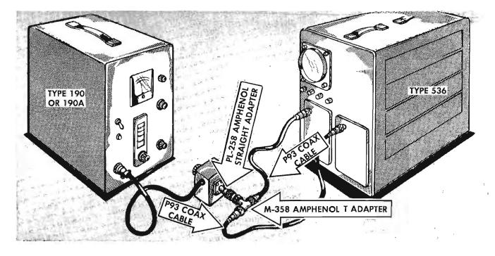
Fig. 6-14. Connecting the Type 190 or 190A Constant-Amplitude Signal Generator to the Type 536.
