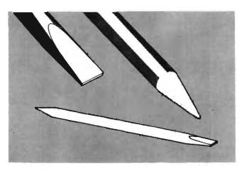
Fig. 5-5. A soldering aid constructed from a 1/4 inch wooden dowel.
