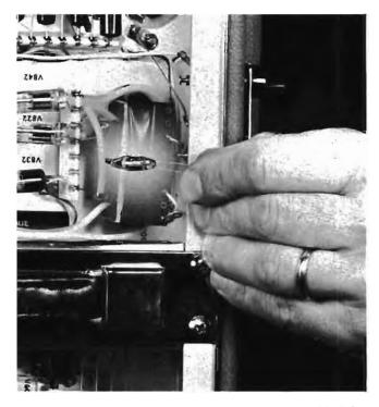
Fig. 5-9. Using a nean lamp to check for energy in the field of the high-voltage transformer.
