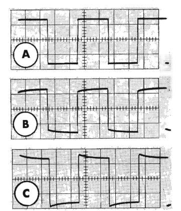
Fig. 6-9. Checking the VERT. SIG. OUT compensation with another oscilloscope.
