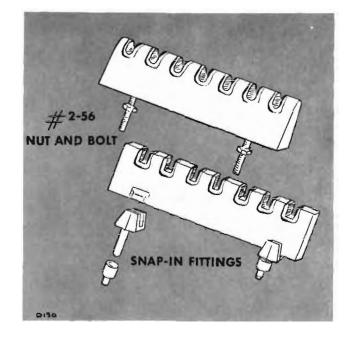
Fig. 5-7. Two types of ceramic strip mountings.
