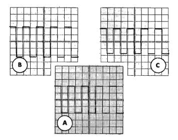
Fig. 6-4. Checking the gain of the vertical amplifier.
