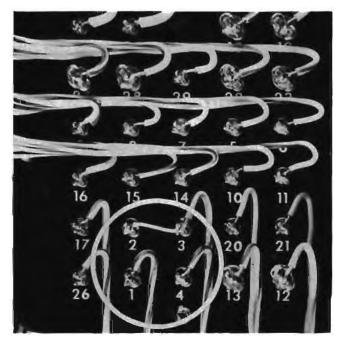
Fig. 3-3. Transformer connections for 234-volt operation.
