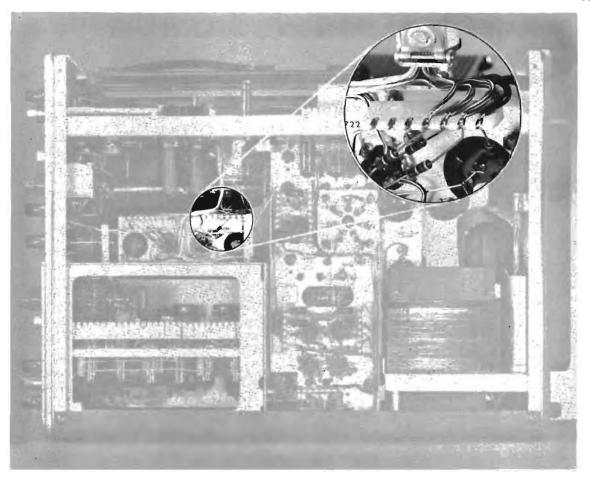
Fig. 5-8. Voltage check points for Low-Voltage Power Supply.
