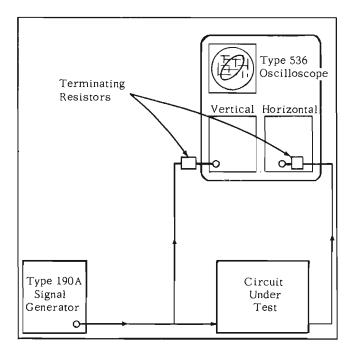
Fig. 3-5. Circuit connections for phase measurements.
