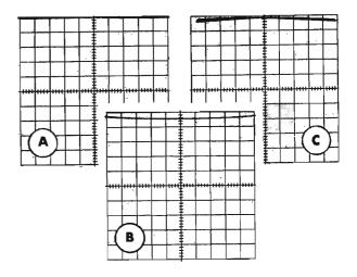
Fig. 6-3. Checking the geometry of the crt.
