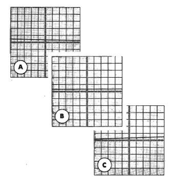
Fig. 6-2. Checking the alignment of the crt.
