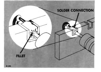
Fig. 5-3. A slight fillet of solder is formed around the wire when heat is applied correctly.
