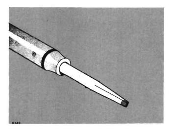
Fig. 5-1. Soldering iron tip properly shaped and tinned.
