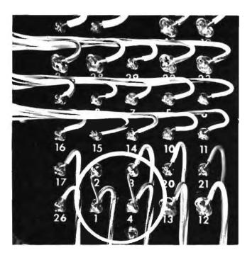
Fig. 3-1. Transformer connections for 117-volt operation.
